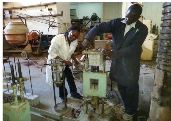
Plate 2: Pull out testing in progress
